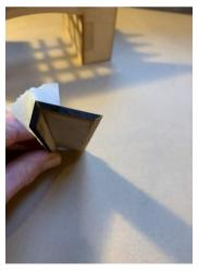
Turn the workpiece over and apply a bead of super-glue down one edge of the vee joint.
