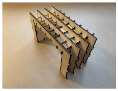
Assemble the internal ribs and spacers ensuring all is square. Assemble 'dry', and then add dabs of superglue once all is in place.
