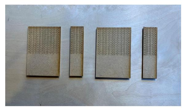
Fold the workpiece up and apply a bead of super-glue down the joins.
