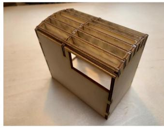
Begin by slotting the pieces of the internal walls together thus: You may find masking tape helpful to hold it all together whilst adding superglue to the internal joins. Set aside to dry making sure it is dead square.
